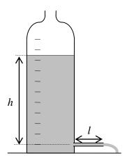
3. <u>Measure the speed *v* of water as a function of the hydrostatic pressure *p*.</u> Fill the bottle and let the water flow. Measure and tabulate the time *t* necessary for
